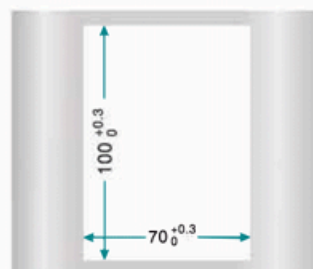
Opening dimension diagram for keyboards without base
