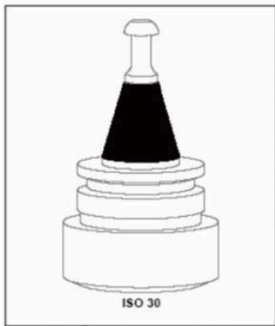
Conical surface of an ISO 30 tool holder (in black)
