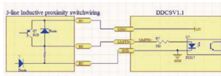
Picture 2-15 Inductive proximity switch wiring mode
