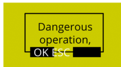
Fig. 6-6 Dangerous prompt for operation of backing to mechanical origin
