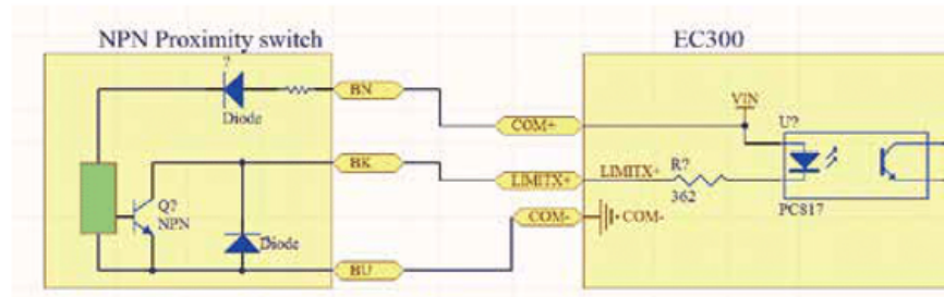
Picture 5-13 Probe/Estop/ and other switch input connection
